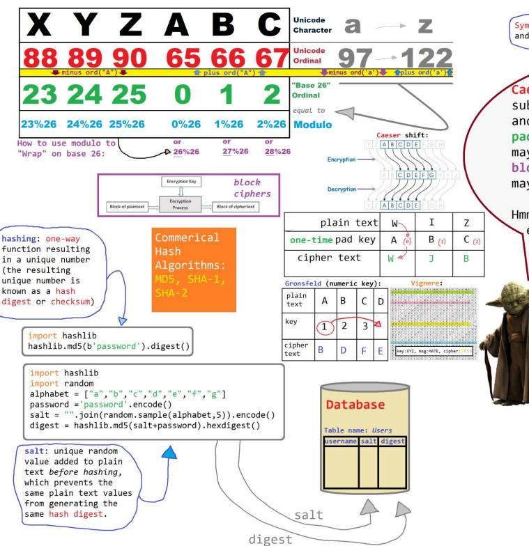
Symmetric cryptography (both encrpytion and decryption) uses the same key
